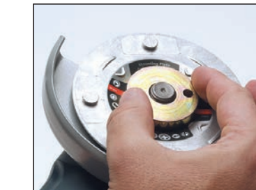
Use your standard locking nut to fasten the backing plate in place. (note: tighten locking nut with spanner wrench. Do not hand tighten)
