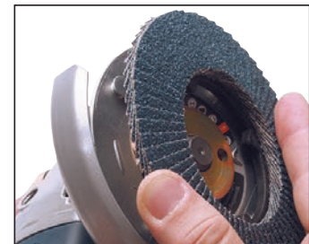
Match the CMT "loading" to the backing plate.
